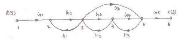
4. Obtain the transfer function using Mason's Gain Formula for the system(MAY/JUNE 2013)
