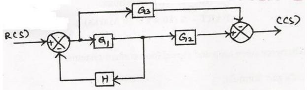
2. Convert the given block diagram to signal flow graph and find the transfer function using mason's gain formula and verify with block diagram approach. (MAY/JUNE 2016)
