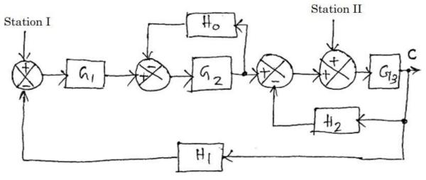
4. Reduce the given block diagram and find the overall transfer function. (APR/MAY 2017) (8 MARKS)
