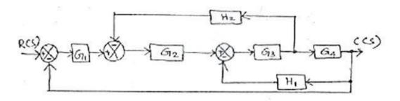
2. Reduce the given block diagram and find the overall transfer function. (NOV/DEC 2014)
