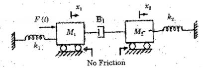
3. Write the differential equation governing the mechanical rotational systems shown in the figure and find the transfer function (**APR/MAY 2017**)
