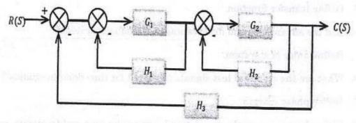
5. Reduce the given block diagram and find the overall transfer function. (APR/MAY 2017) (8 MARKS)
