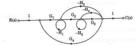
6. Obtain the transfer function using Mason's Gain Formula for the system(APR/MAY 2017)  $H_1$   $H_2$
