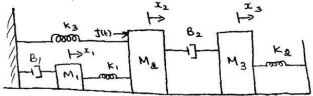
**3.** Write the differential equation governing the mechanical translational systems shown in the figure. Draw the Electrical analogous circuits. (MAY/JUNE 2013)
