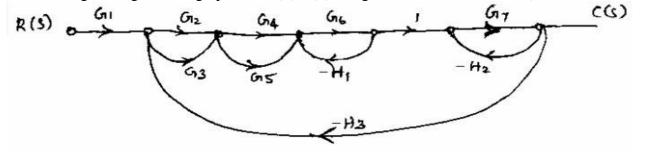
2. For the given signal flow graph find C(S)/R(S) using Mason's Gain formula. (NOV/DEC 2013, APR/MAY 2017)
