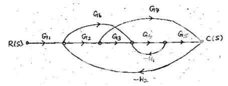
3. For the given signal flow graph find C(S)/R(S) using Mason's Gain formula. (NOV/DEC 2013)
