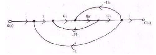
5. Obtain the transfer function using Mason's Gain Formula for the system(APR/MAY 2017)
